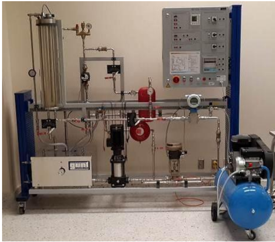
Fig Lab E007: Gunt 4-Variable Process Control module
